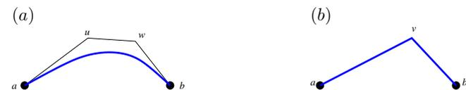
Figure 4: (a) A Bezier curve segment. (b) A corner segment
